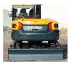
Compact and appealing design The HX85A has been designed with a short rear swing radius for a perfect fit in narrow jobsites requiring high flexibility.
