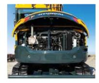
Engine hood The large rear engine hood opens wide to provide easy access for maintenance tasks.
