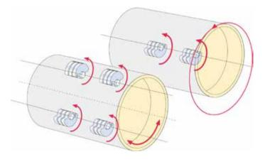
The Dynapac CO4000 VI, CO4200 VI and CO5200 VI rollers have one vibrating drum with two vibration amplitudes and one oscillating drum. This allow the operator to select the system that is most suitable for the application on hand. High wear resistant Hardox drum shell
