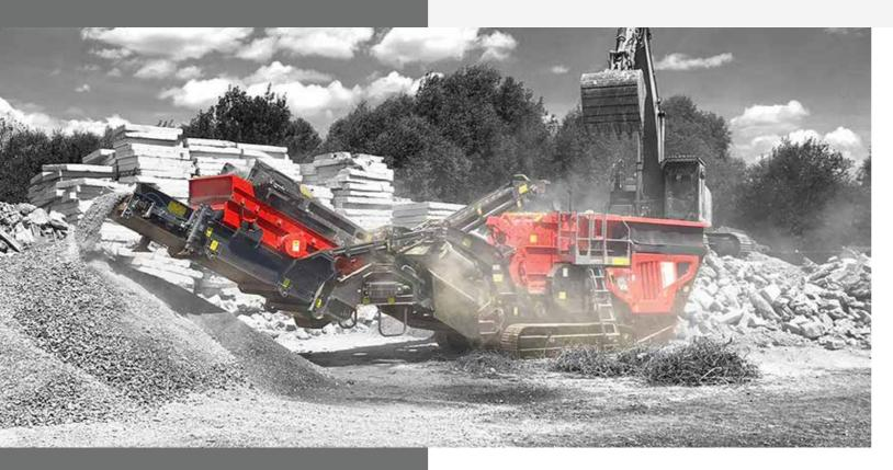
The Finlay® IC-110RS mobile impact crusher provides the versatility of a compact crushing and screening plant on one mobile platform for quarrying, construction and demolition debris, reinforced concrete and asphalt recycling applications. The machine features a direct drive Ø1034 x 1000mm (Ø41.5" x 40") horizontal impact crusher with variable speed control to give operators unprecedented levels of fuel efficiency and productivity.
