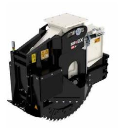
Intended for excavator boom mounting, they are specially indicated for **cutting and narrow trenching for fiber** optics installation on hard and compact surfaces: asphalt, concrete and rock. Slides parallel to the ground. Constant trenching depth. Mechanical or hydraulic adjustment of trench depth.
