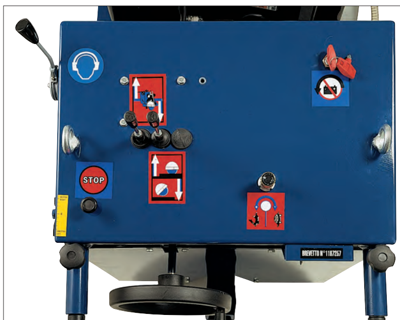
VDAI Saw: view of control panel with automatic forward/backward advancement lever; lever for lowering and raising the cutting blade; knob for adjusting the advancement speed and other controls. This photo shows the handwheel of the mechanical drive control device.
