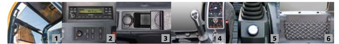
1 Roller shade 2 Radio & USB player with remote control 3 Hands-free cell phone 4 Joystick 5 Accel dial with LED lamp 6 Storage compartment
