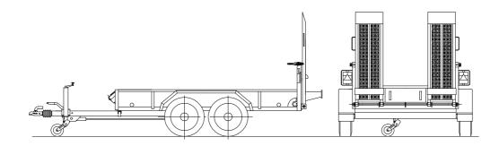
Axles: Maintenance-free rubber spring axles with precision bearings
