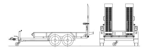
Axles: Maintenance-free rubber spring axles with precision bearings
