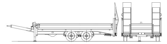
Axles: Fast-running BPW axles with S-cam brakes, maintenance-free parabolic spring assembly and weight
