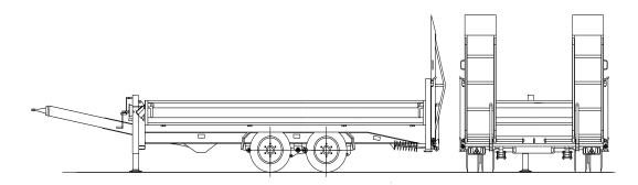
Axles: Fast-running BPW axles with cam brakes, maintenance-free parabolic spring assembly and weight adjustment
