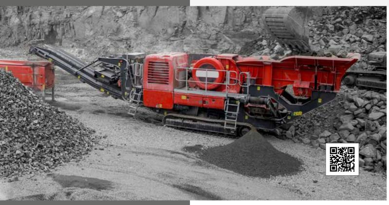
The Finlay® J-1160 primary mobile jaw crusher was designed with the customer and operator in mind. The new model features increased under jaw clearance and all round preventative maintenance and serviceability access.
