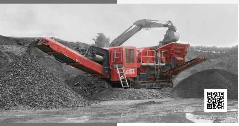
The Finlay® J-1175 mobile Jaw Crusher is a high performance and aggressive primary crushing plant for medium sized operators in quarrying, demolition, recycling, and mining applications.
