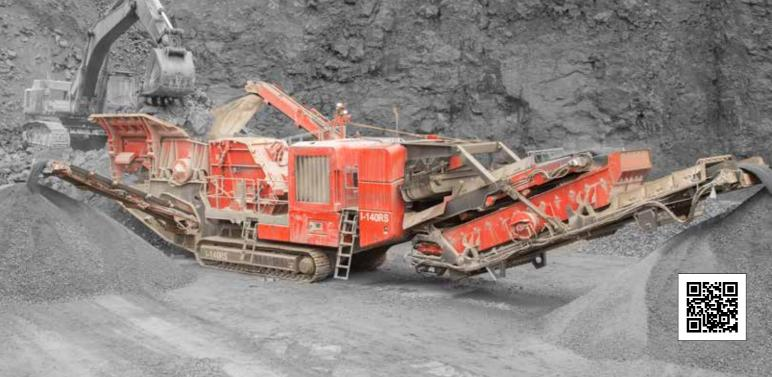
The Finlay® I-140RS mobile impact crusher has been designed to give improved material flow and production capabilities in quarrying, mining, demolition and recycling applications.
