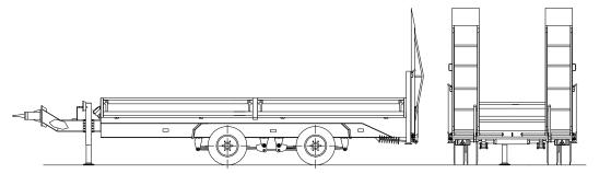
Axles:Fast-running axles type Gigant with cam brakes, maintenance free air suspension with lifting and lowering;<br/>distance of the axles about 1,80m
