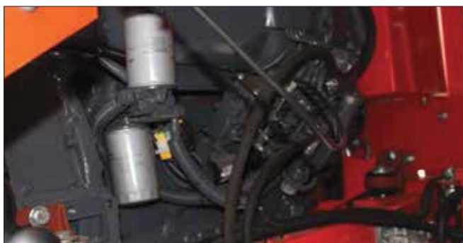
Engine: Tier 3 / Stage IIIA Deutz D914 L04i
