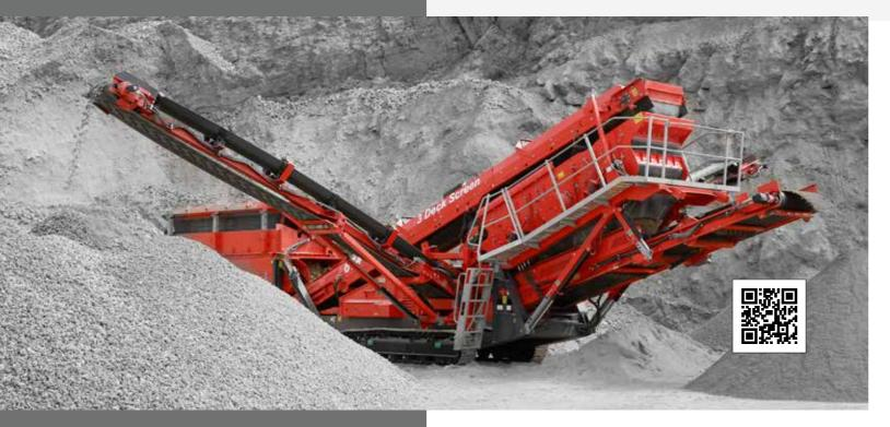
The Finlay® 674 inclined screen is a compact easily transportable machine that offers operators rapid set up and tear down times. The screenbox features three decks giving a large screening area of 170ft² to provide efficient screening even at small fractions and high capacity.
