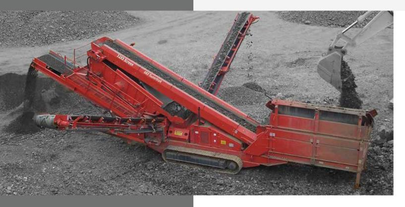
The Finlay<sup>®</sup> 683 inclined screen is ideally suited for small to medium sized operators and contractors who require a versatile product capable of operating in a number of applications such as sand and gravel, aggregates and recycling.
