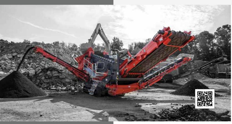
The Finlay® 883+ Spaleck mobile recycling screen is the ultimate in mobile screening and separation technology. At the heart of the screen is the two deck German designed and constructed high performance recycling waste screen with Flip-Flow-Screen Elastica.
