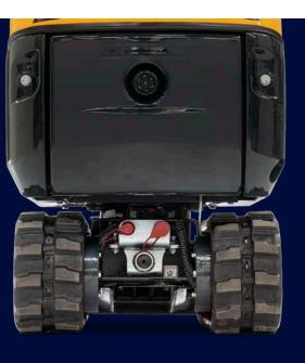
An external hydraulic oil tank keeps oil cooler without an additional cooling system. This protects performance in high ambient temperature.
