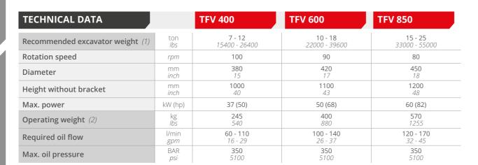
(1) User is responsible for ensuring that the equipment meets the excavator's specifications and weight requirements. (2) Without mounting bracket attaching to prime mover.
