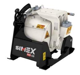
Designed to **mill pre-set** sections on hard and compact surfaces, the PLB and PHD planers for excavators are able to remove the entire layer of asphalt or concrete in preparation for trenching, or are used to mill deteriorated sections for later resurfacing.
