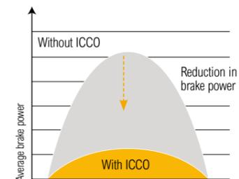
The **Intelligent Clutch Cut-Off (ICCO)** function minimises loss of power in the torque converter and prevents excessive power use during braking. This reduces heat generation and wear on the brake disc.
