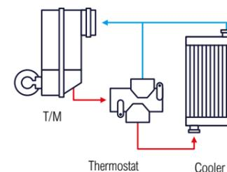
The HL960A is equipped with a **thermostat for transmission cooling**. This feature helps to warm up the fluid quickly and keeps it at the optimal working temperature in winter, protecting components and increasing efficiency.
