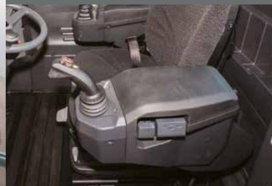
The HL960A has a **large comfortable seat** with heating as standard. The seat and armrest are fully adjustable and, for added comfort, an air suspension version is available as an option. Thanks to the **electro-hydraulic implement control lever**, less force is needed to operate attachments, helping you to work longer and more productively.
