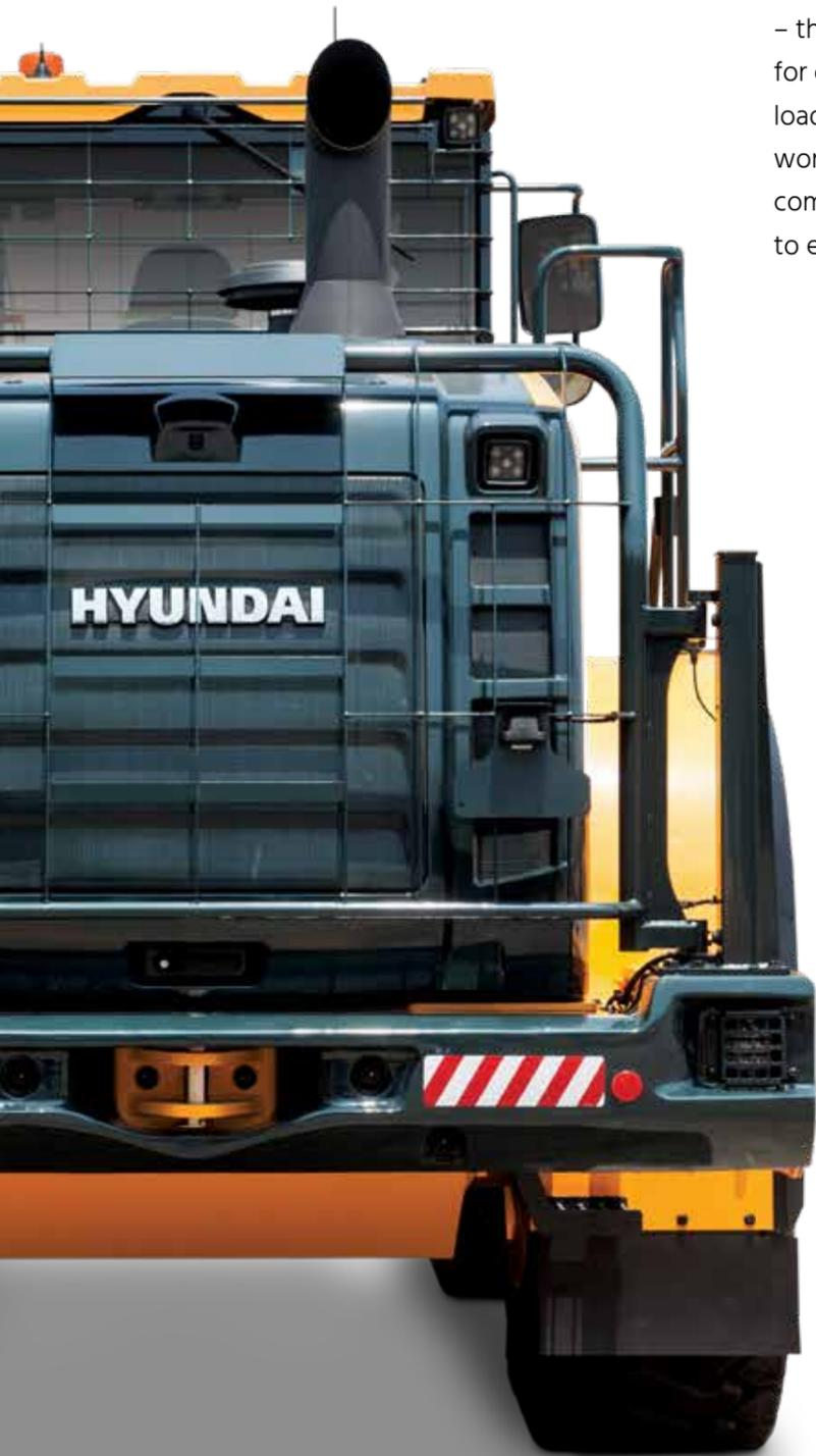
▶ A **rear grill guard** protects the rear-view camera, work lights, license plate lamp and radiator from falling debris. The design does not impede the operator's view. The steel guard is hinged and opens to allow easy access to the radiator for cleaning or daily maintenance.
