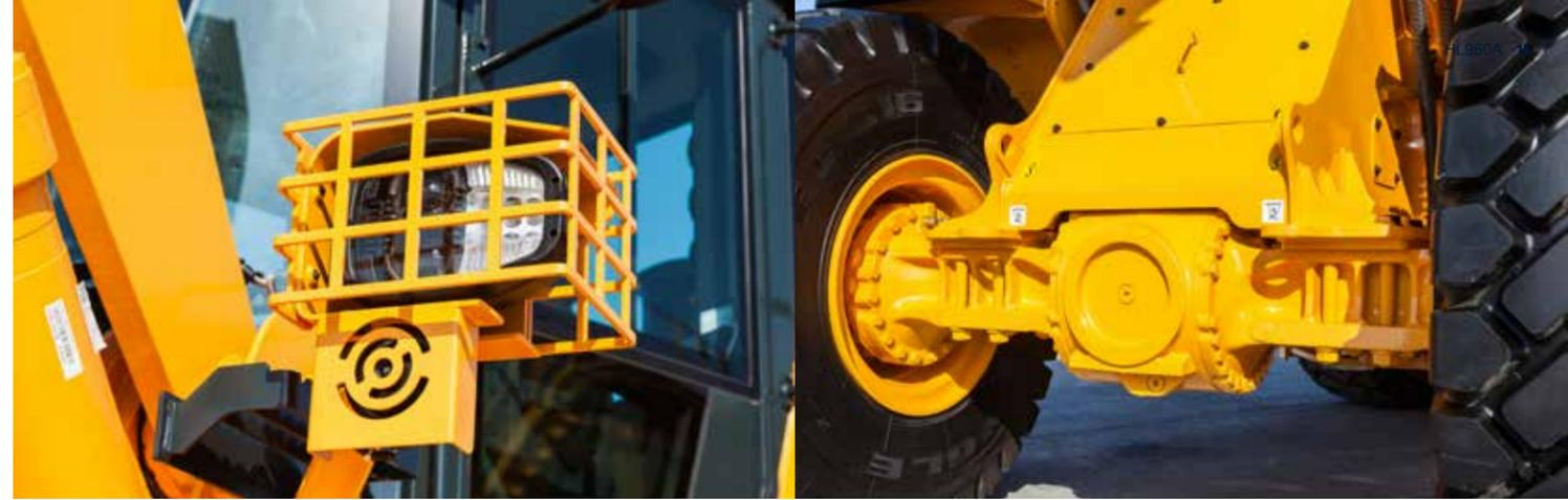
▶ A **steel grill housing** protects the front and rear working lights from material spill from the bucket.
