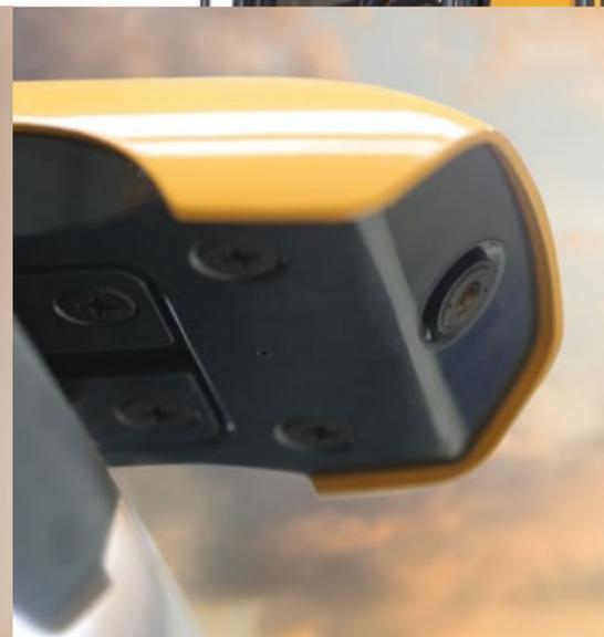
The optional **Advanced Around View Monitoring (AAVM)** system gives you a 360° overview of your immediate working environment. It also includes Intelligent Moving Object Detection (IMOD) technology that senses and warns you when people or objects come within five metres of the machine.
